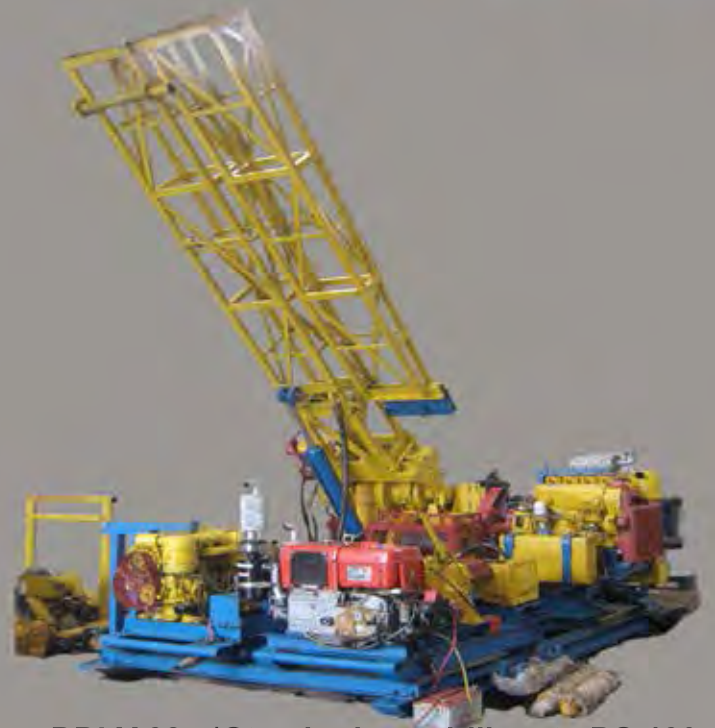
DDLY 38 - *Standard can drill up to PQ 130m, HQ 300m, NQ 400m, while *Modified can drill up PQ 250m, HQ 450m & NQ 650m
