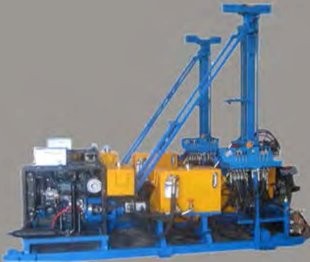
DDJC250 can drill up to PQ 150m, HQ 250m and NQ 300m
