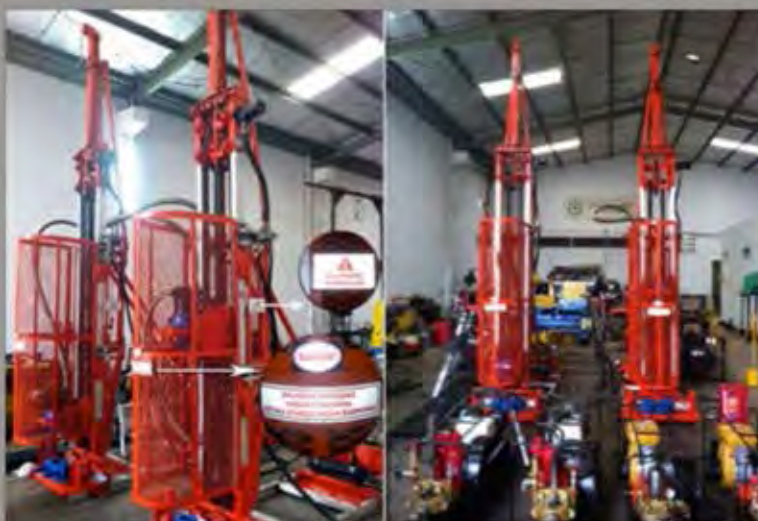
DDJC175 can drill up to HQ Open Hole 120m (Single Tube) & HQ Coring 80m (Triple Tube)
