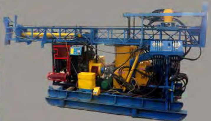
DDJC500 (Modified Engine+Hyd Pump) can drill up to PQ 200m, HQ 350m and NQ 500m
